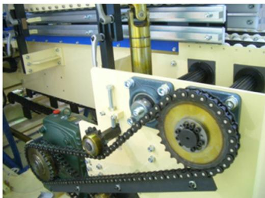
**Figure 2 Drive components of conventional packaging machine**
