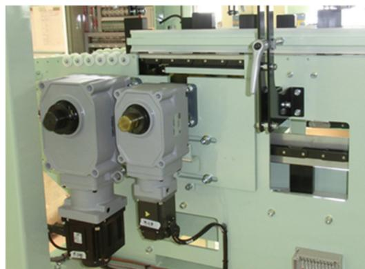
**Figure 3 Drive components of new packaging machine**
