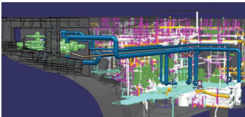
**Figure 1** Example of repair engineering - Ballast water management system installation
