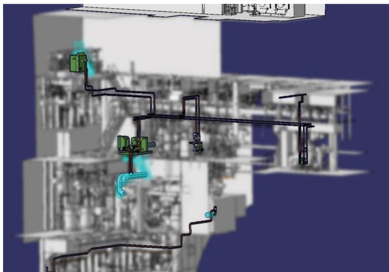
**Figure 3** As-Built 3D CAD model with the repair area appended (starboard side of VLCC)
