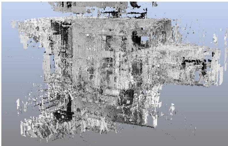
**Figure 2** Point cloud data acquired by 3D laser scanner
