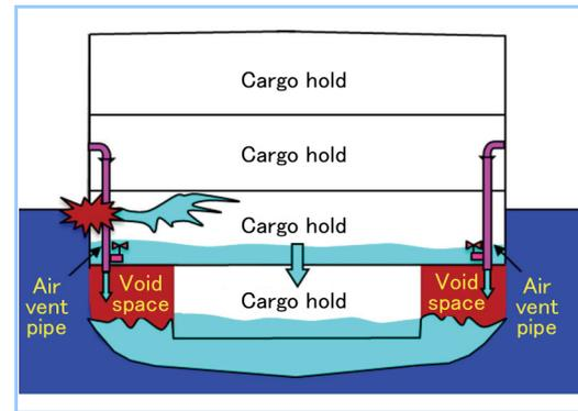
Figure 3 Downflooding through air vent pipes
