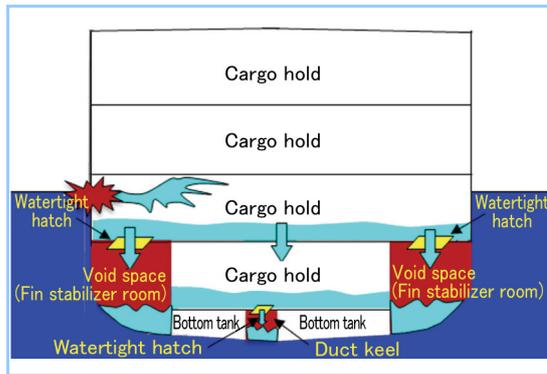
Figure 2 Downflooding through watertight hatches
