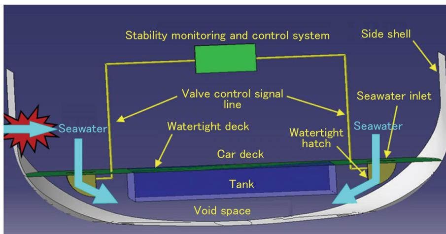
**Figure 1** Conceptual drawing of stability recovery system
