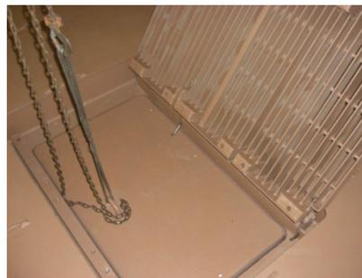
**Figure 5** Downflooding hatch at the lower car deck
