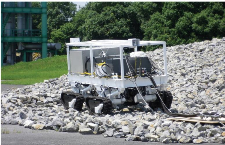
**Figure 5 Element test for the crawler device**
