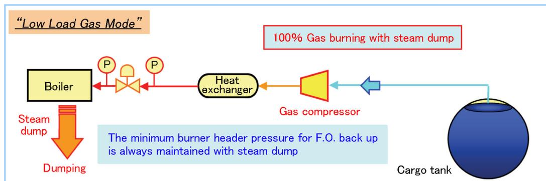
Figure 2 Overview of Low Load Gas Mode (LLGM)
