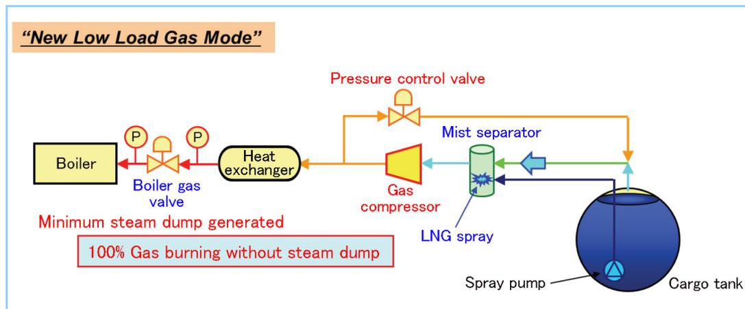
Figure 4 Overview of New Low Load Gas Mode (NLLGM)
