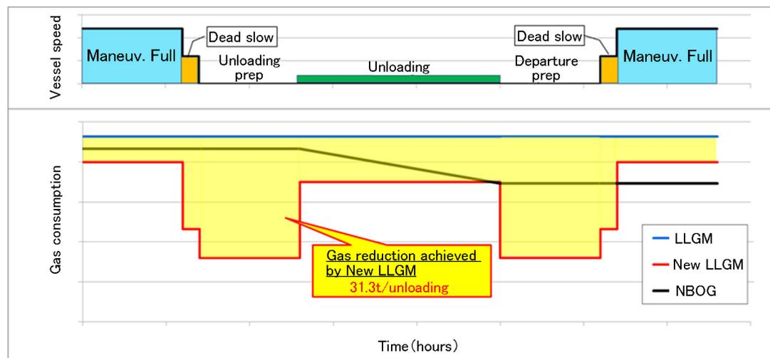
Figure 5 LLGM vs. NLLGM performance comparison: unloading
