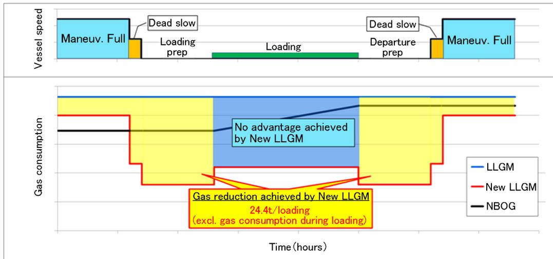
**Figure 6 LLGM vs. NLLGM performance comparison: loading**
