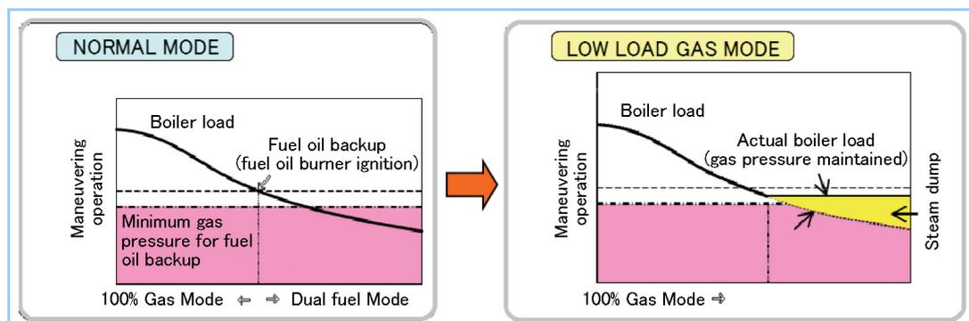
Figure 3 Comparisons: Boiler load and fuel mode
