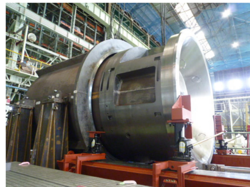
Figure 9 Bundle pull-out test in plant
