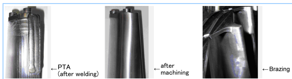
Figure 18 Stellite coating on final stage blades
