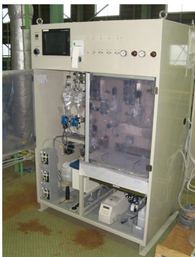
Figure 8 Photograph of the online measurement device for absorption solvent
