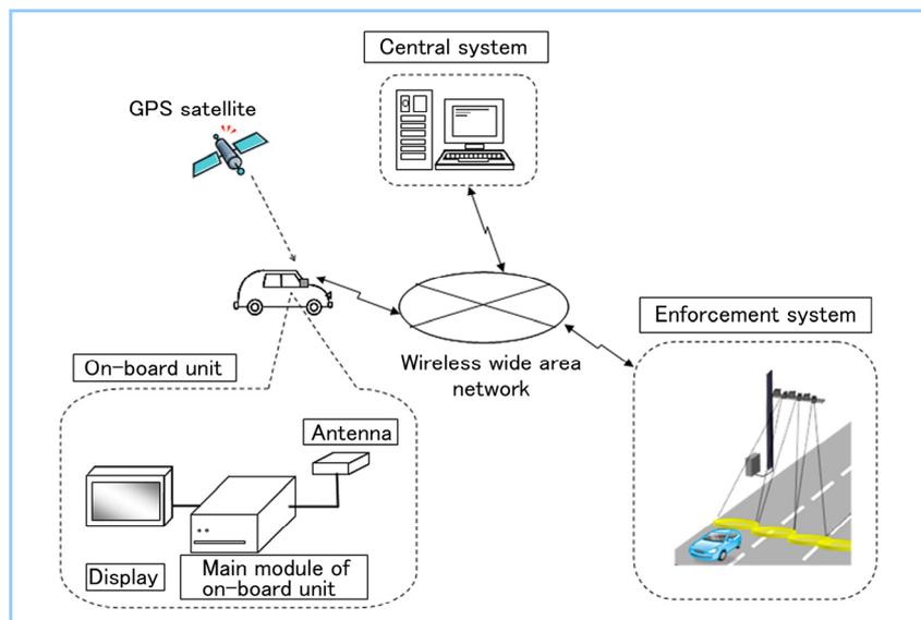
Figure 1 Configuration of MHI's GPS-based ERP system
