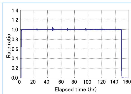
Figure 8 Long-term stability of film deposition rate
