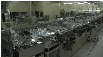
Figure 5 Overview of the in-line deposition system
