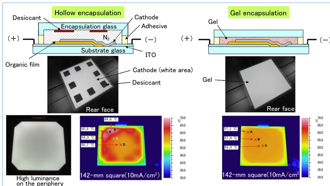
Figure 4 Emission state of panel and heat generation (when lighting at 5,000 cd/m<sup>2</sup>)
