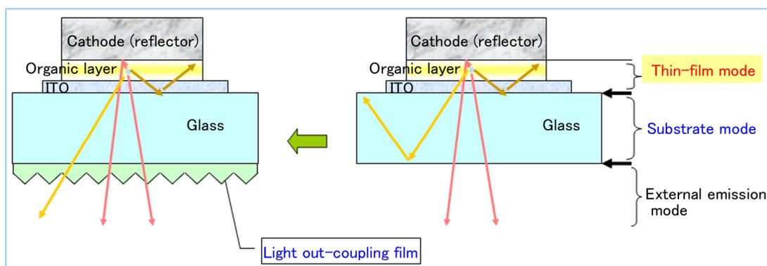
**Figure 3 Light propagation mode of OLED devices and effects of the light out-coupling film**
