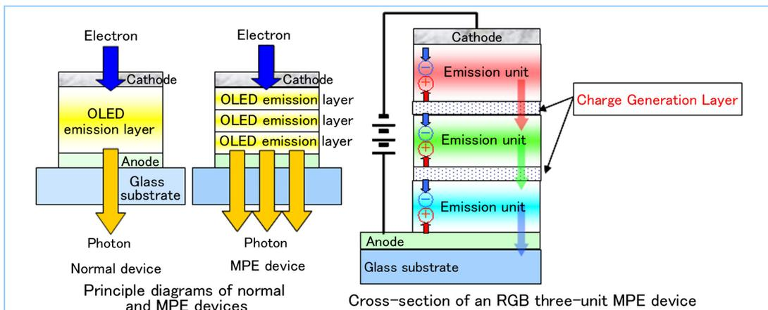
**Figure 1** Principle and cross-sectional diagrams of multi-photon emission devices
