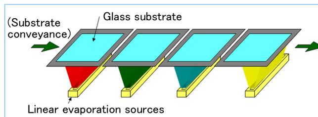
Figure 6 Schematic diagram of linear evaporation sources and in-line conveyance
