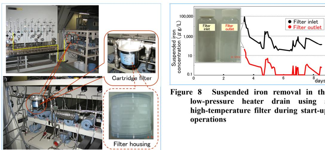
**Figure 7** External view of the suspended iron removal test unit with a high-temperature filter for the low-pressure feed-water heater drain system
