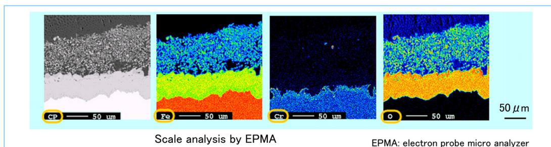
Figure 5 Powdered scale deposited on the boiler generating tube
