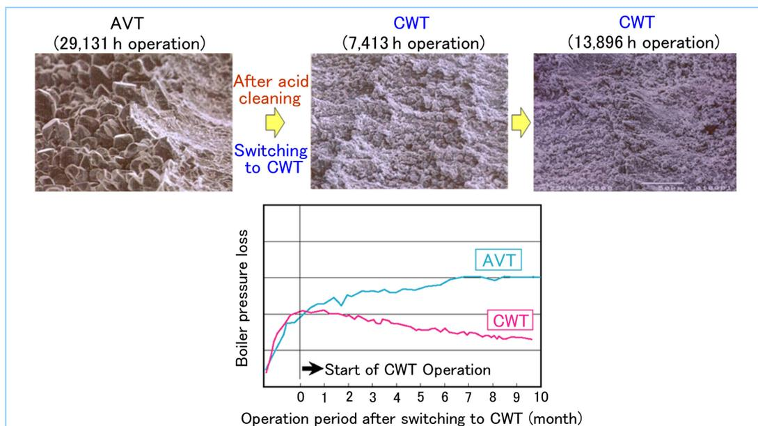
Figure 3 CWT effect of reduced rippled scale build-up
