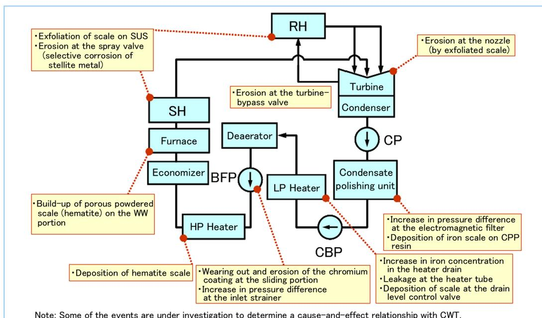
Figure 4 Example problems at inspected CWT plants
