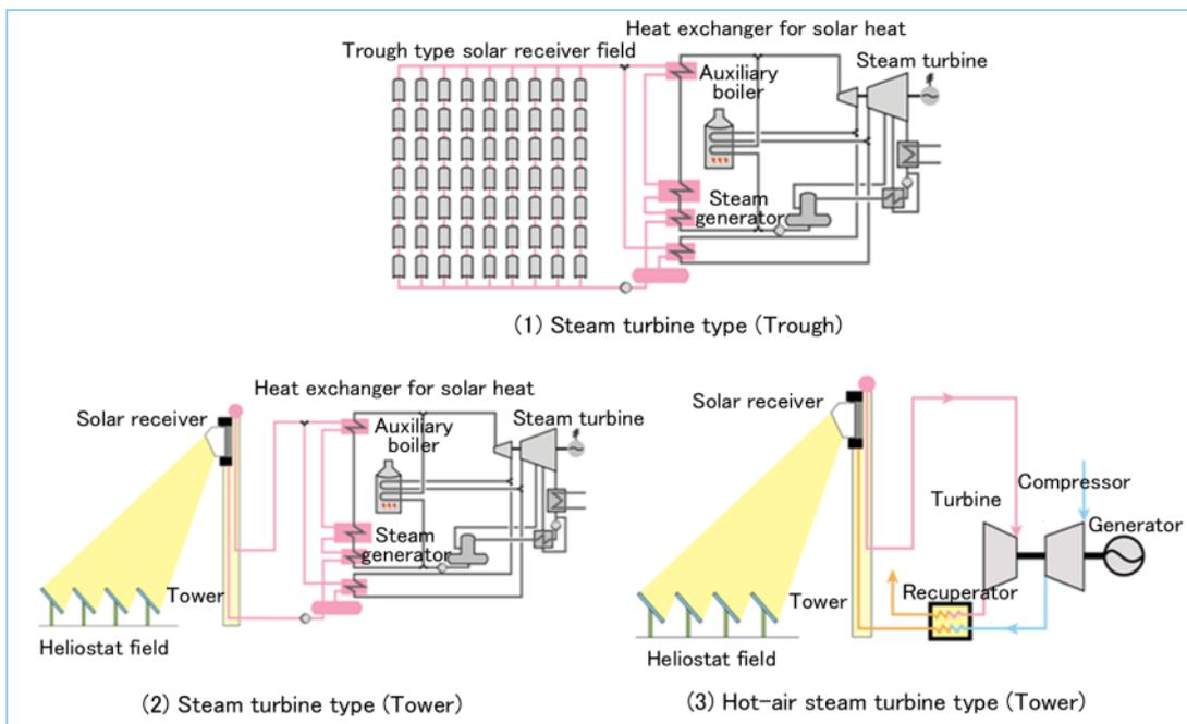
**Figure 3 Comparison of concentrated solar power generation systems**
