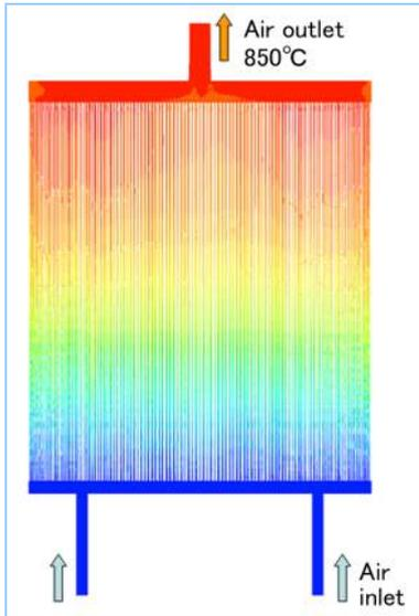
**Figure 4 Results of three-dimensional heat radiation analysis (air temperature distribution)**
