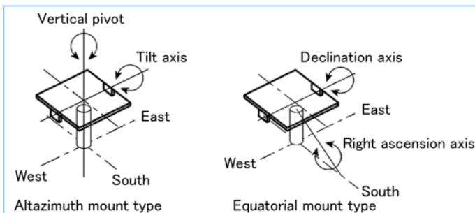
**Figure 6 Examples of heliostat construction**
