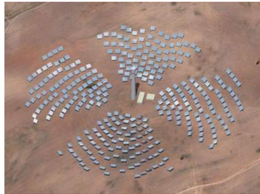
**Figure 8 Plant image showing heliostat arrangement**
