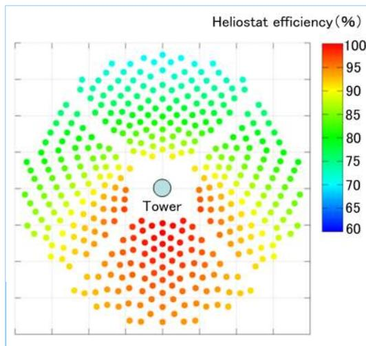
**Figure 7 Example of a heliostat efficiency evaluation**
