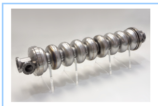
Figure 1 Superconducting accelerating cavity intended for ILC R&D (Courtesy of KEK)
