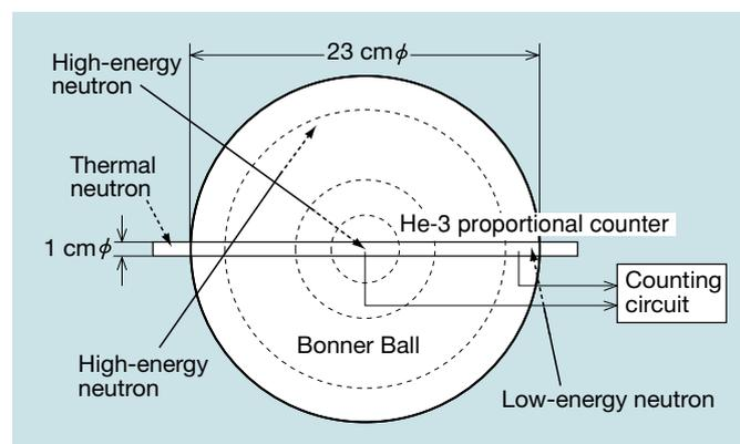
Fig. 1 Measurement principle of a single-sphere-type Bonner Ball detector
