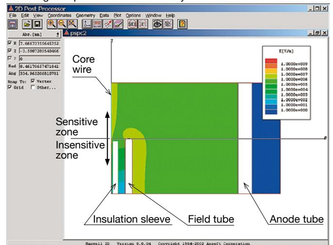
Fig. 5 Analysis of the electric field in the proportional counter (applied voltage of 2 kV)
