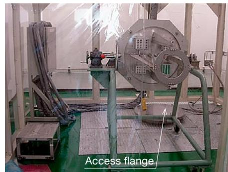
**Fig. 5 Clean booth used for the thruster setting at the combustion test facilities**
