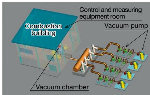
(b) 3 dimensional view of the combustion test facilities
