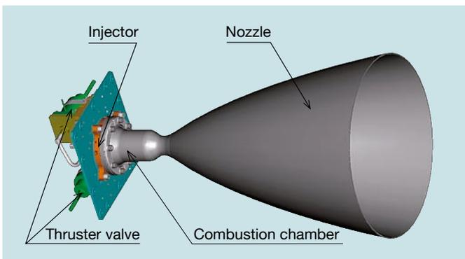
**Fig. 1 Thruster configuration**
