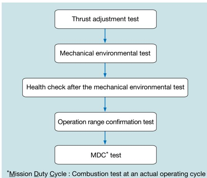
**Fig. 7 Qualification test flowchart**
