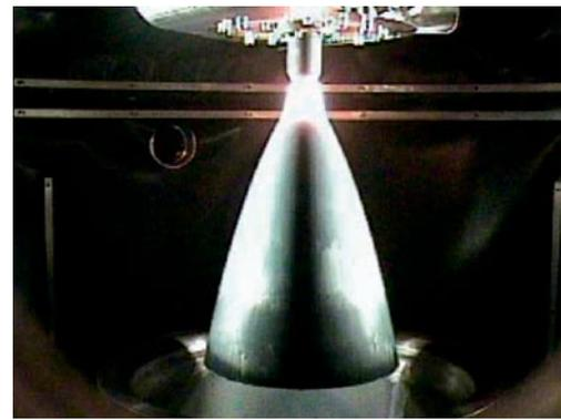
**Fig. 8 500N ceramic thruster setup in the vacuum chamber during the thrust adjustment test**
