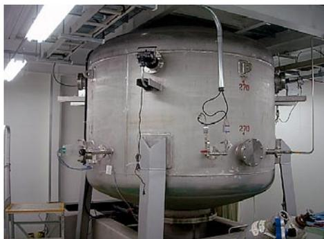
**Fig. 4 Vacuum chamber used for the combustion test facilities**
