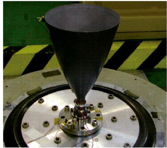
**Fig. 9 Setup of the mechanical environmental test with the 500N ceramic thruster fixed on the vibrator**
