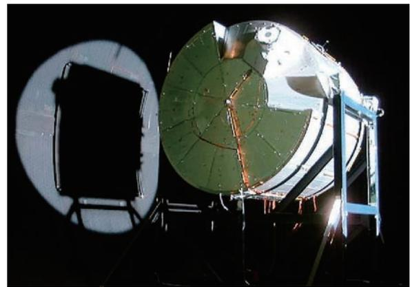
Fig. 4 ELM-PS thermal balance test (Courtesy of JAXA)
