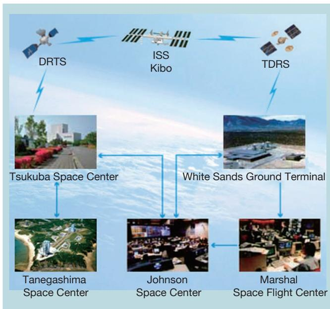
**Fig. 6 Overview of the Kibo operations system (Courtesy of JAXA)**
