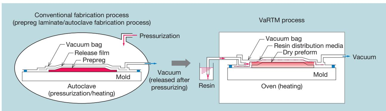
**Fig. 1 Differences between composite fabrication processes**
