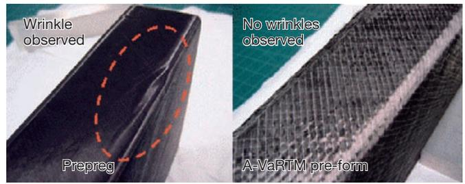
**Fig. 2 Comparison between A-VaRTM pre-form and prepreg**
