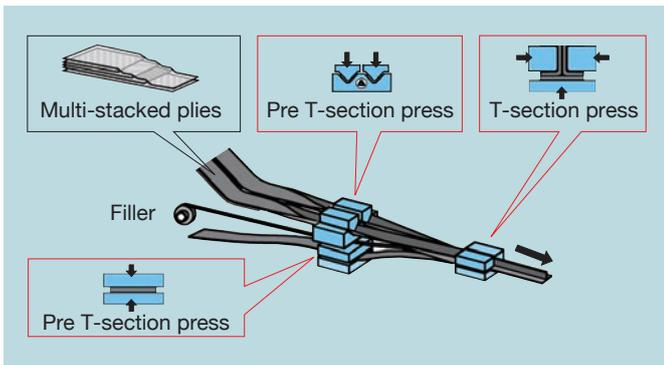
**Fig. 4 Automatic press forming for a T-section stringer pre-form**
