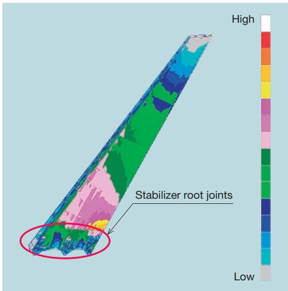
**Fig. 7 Strain distribution of strains determined by FEM analysis**
