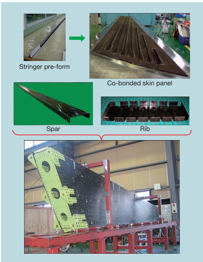
**Fig. 5 Full-scale vertical stabilizer test specimen**
