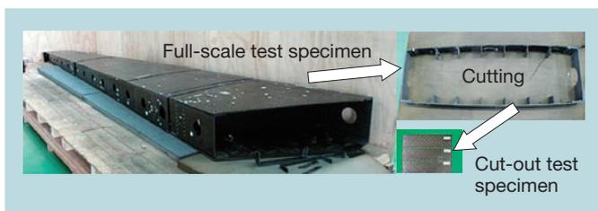
**Fig. 8 Cutting the full-scale test specimen**
