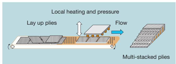
**Fig. 3 Schematic diagram of automatic multi-stacking**
