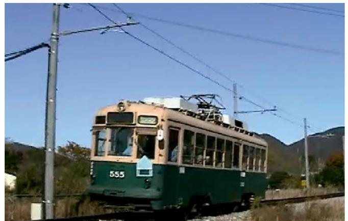
Fig. 5 Operational testing of a battery-powered LRT vehicle
