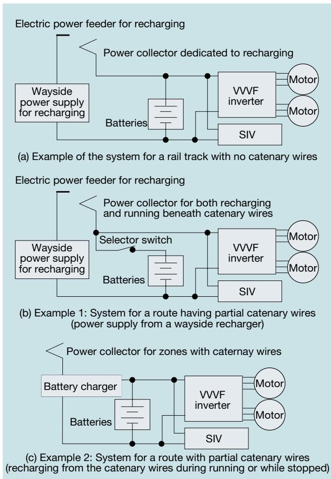
Fig. 3 Examples of system configurations for battery-powered LRT
