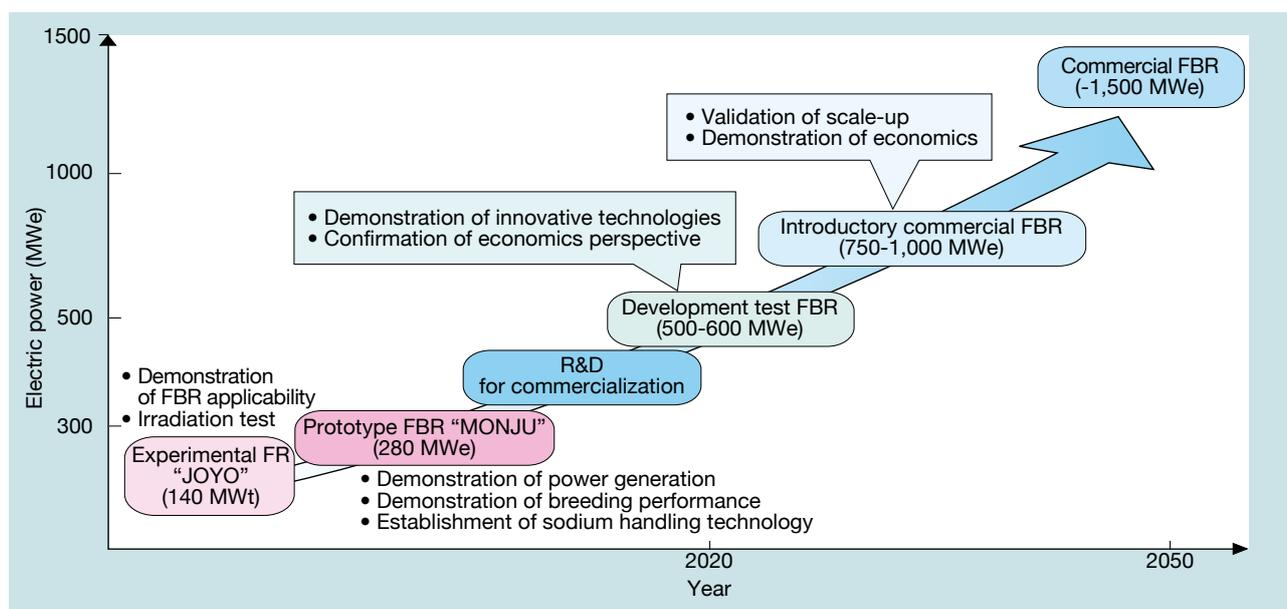
Fig. 3 Conceptual Road Map for the Development of Commercial FBR<sup>8</sup>
