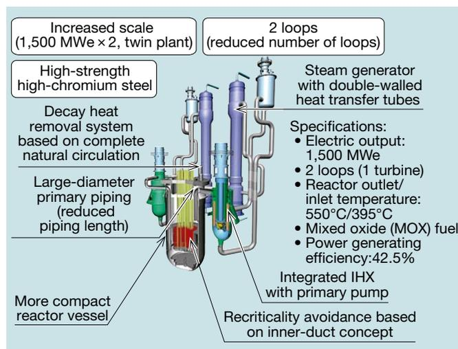
Fig. 2 Sodium-Cooled Loop Type Large-Scale FBR<sup>4</sup>
