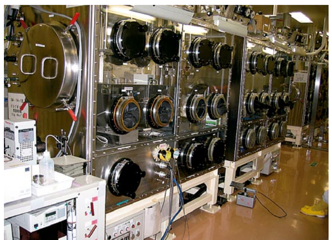
Fig. 3 Outward Appearance of Direct Extraction Test Equipment 7 Former JNC/Test equipment installed inside the CPF glove box
