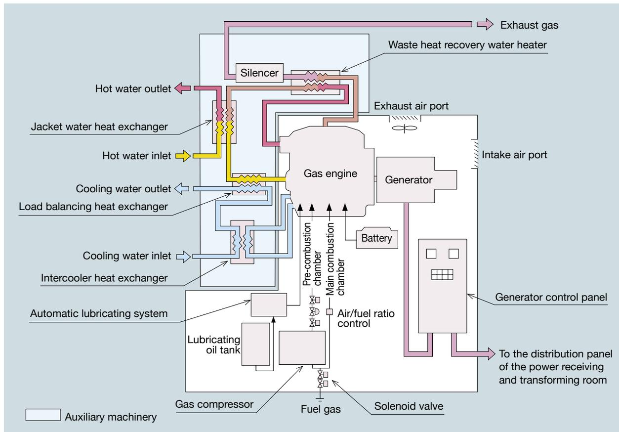
**Fig. 5 Block diagram of the hot water recovery system**
