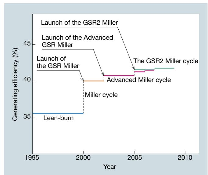
Fig. 1 History of MHI's improvement of gas engine efficiency
