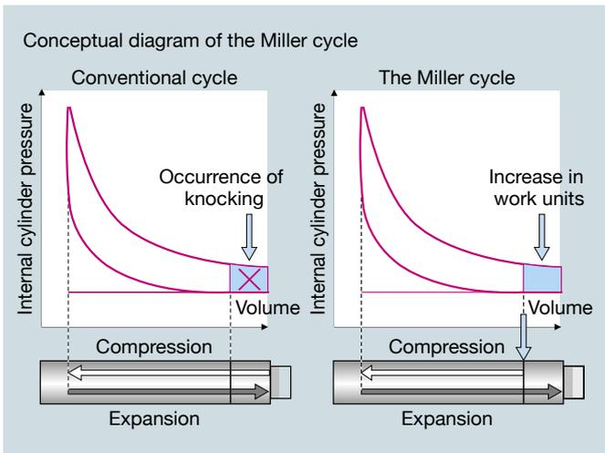
**Fig. 2 Conceptual diagram of the Miller cycle**
