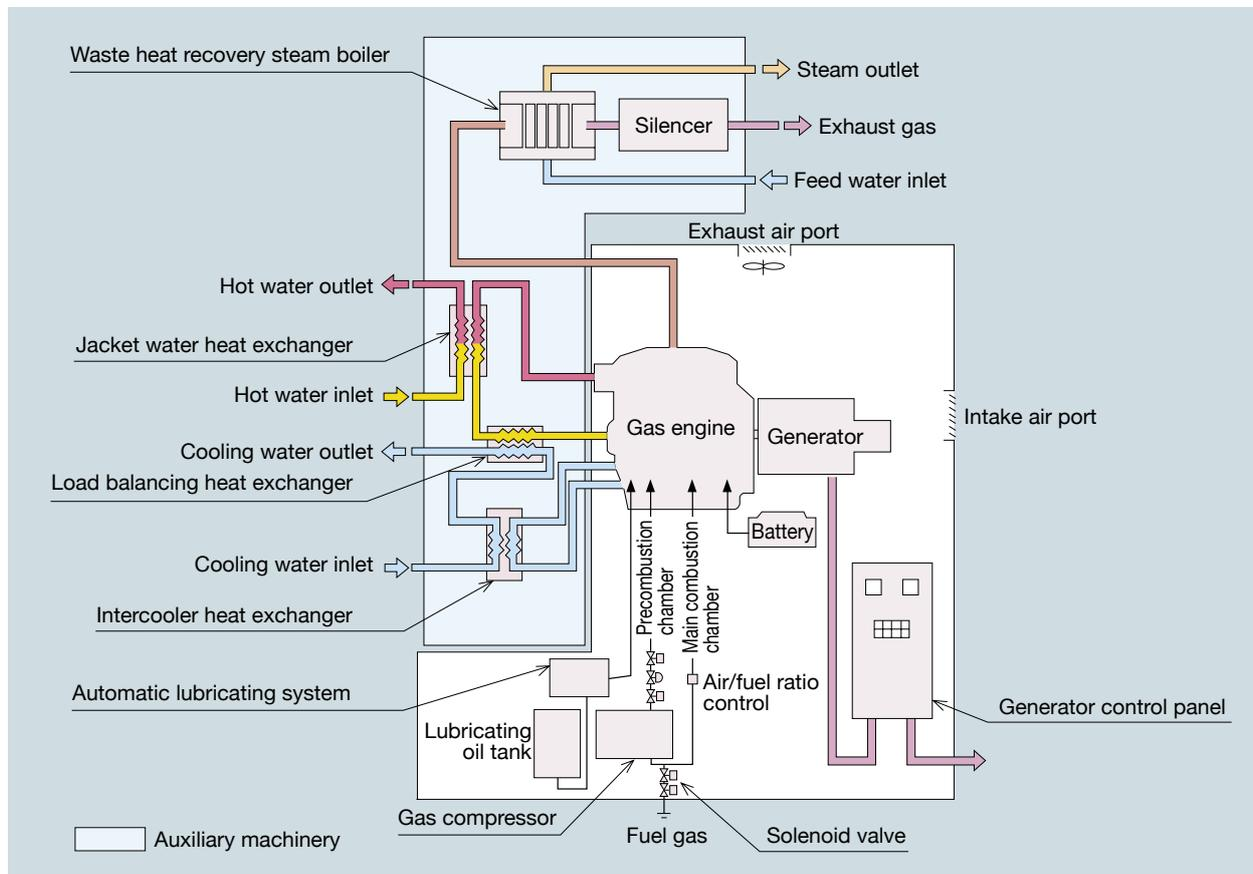
**Fig. 3 Block diagram of the hot water and steam recovery system**
