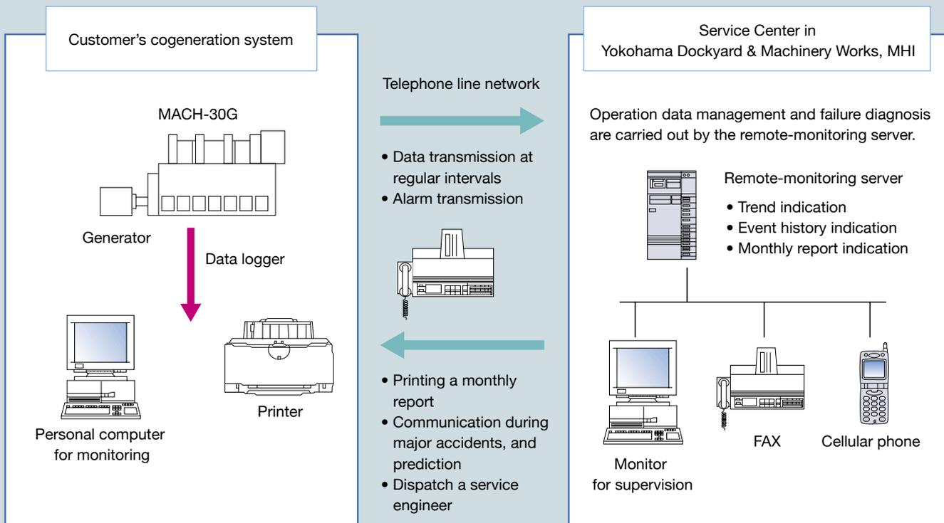
**Fig. 4 Remote monitoring system**
