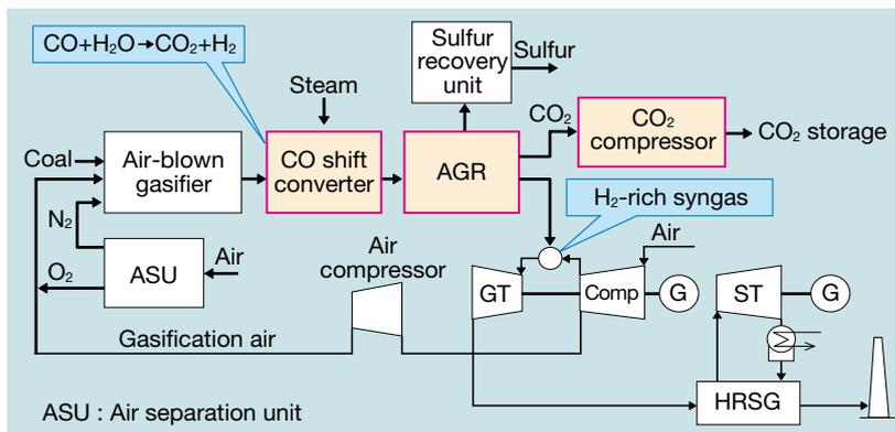
**Fig. 2 Block flow diagram of the air-blown IGCC system with CO<sub>2</sub> capture**
