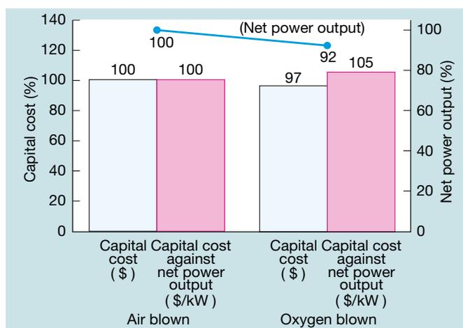
**Fig. 3 Comparisons of capital cost and net power output between the air-blown IGCC and oxygen-blown IGCC during CO<sub>2</sub> capture**
