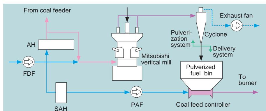
Fig. 2 Bin system (indirect combustion system)
