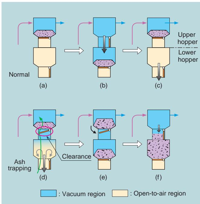
Fig. 13 Lock hopper ash conveying system
