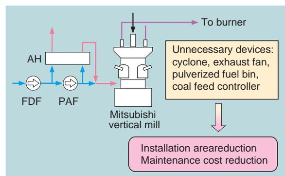
Fig. 3 Direct mill system (direct combustion system)
