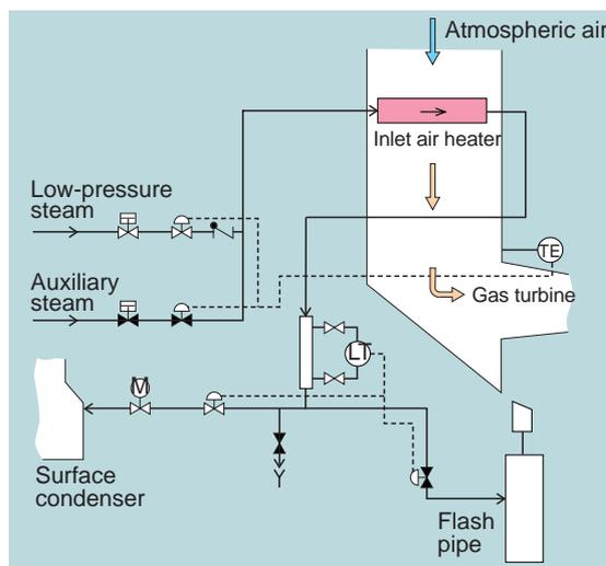
Fig. 5 Outline schematic of inlet air heating system
