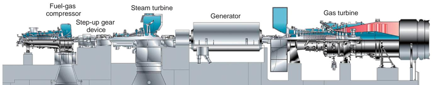
**Fig. 3 Longitudinal sectional drawing of complete assembly**
