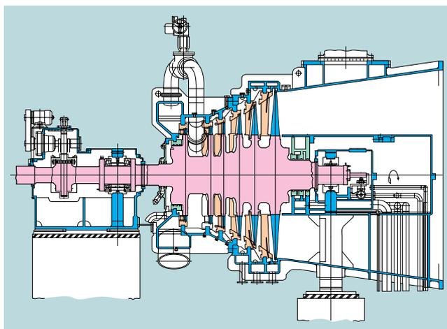
Fig. 2 Turbine sectional assembly
