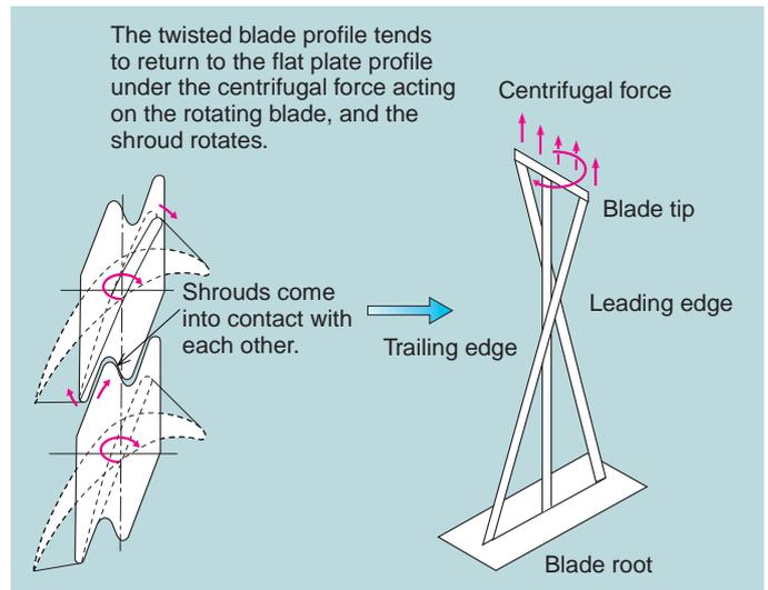
**Fig. 7 Contact status of ISB shrouds during operation**
