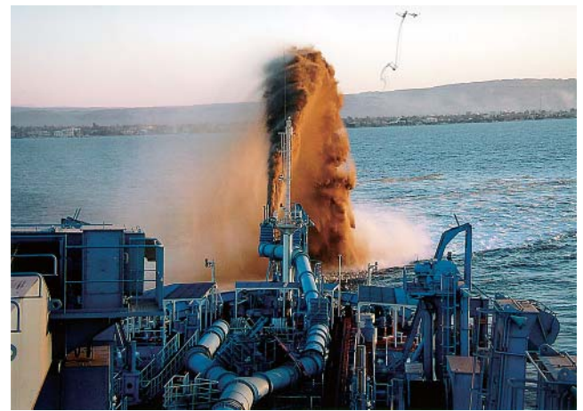
Fig. 2 Discharging by bow discharge nozzle (Rainbow)
