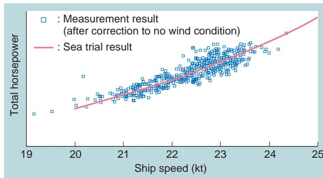
**Fig. 12 Ship speed-brake horsepower curve (correction to a no-wind condition)**
