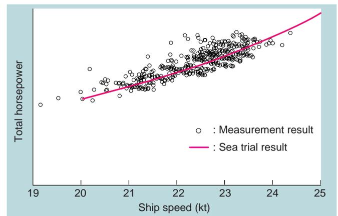
**Fig. 9 Ship speed-brake horsepower curve (measurement result)**
