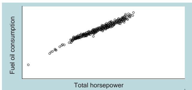
**Fig. 8 Relation between brake horsepower and fuel oil consumption**
