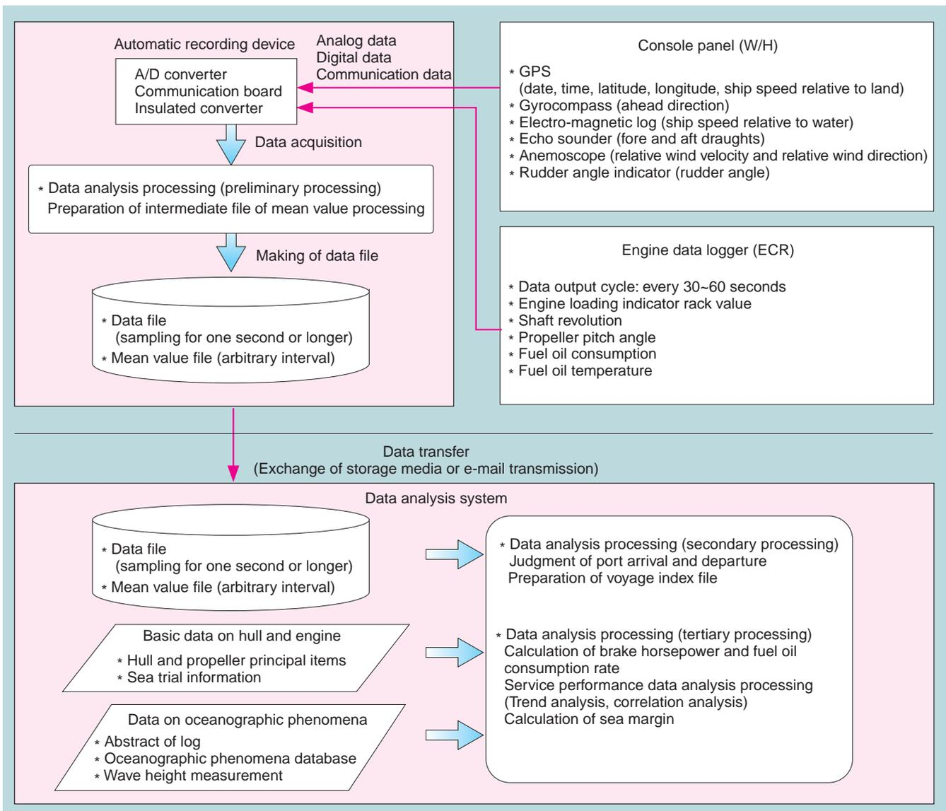
**Fig. 1 System configuration scheme**
