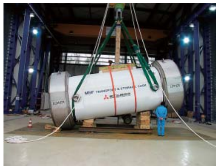
Fig. 11 Full scale drop test model (MSF-69B) At the BAM drop test facility in Horstwalde, Germany.
