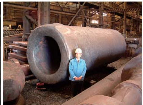
Fig. 9 Fabrication of the main body shell of the cask by the monolithic forging method
