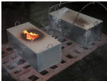
Fig. 7 Fire testing for the neutron shielding Verification of the self extinguishing ability after fire testing at 800°C x 30 minutes.
