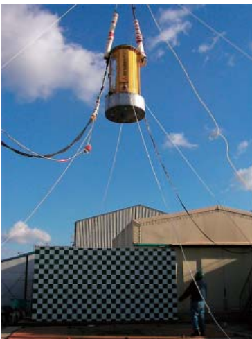
Fig. 10 9 m drop test with 1/2.35 scale drop model In-house drop test site in the Takasago Research & Development Center.
