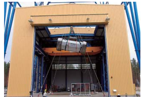
Fig. 12 Certification test with full scale model At BAM drop test facility in Horstwalde, Germany.
