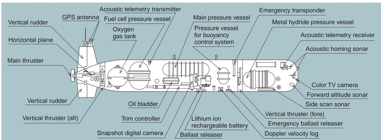
Fig. 1 General arrangement of vehicle Configuration and layout of the vehicle (side view)
