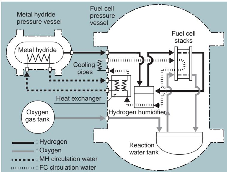
**Fig. 2 Block diagram of fuel cell system**
