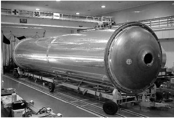
Fig. 2 Rocket propellant tank appearance The figure shows the appearance of the current H-IIA rocket first stage liquid hydrogen tank as a representative example of rocket tank.
