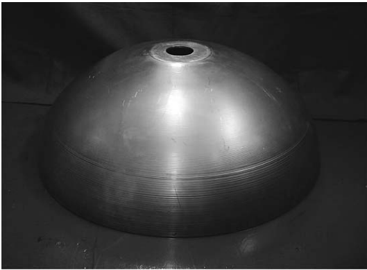
Fig. 8 Dome produced on an experimental basis (diameter 900mm) A sub-scale dome was produced on an experimental basis by spin forming.
