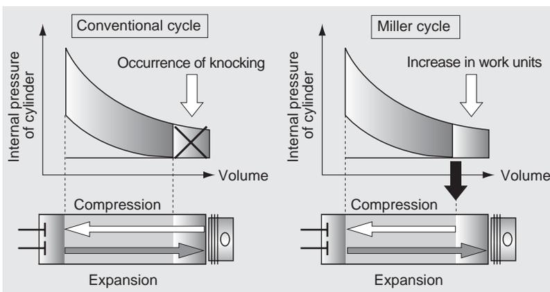
**Fig. 3 Concept of the Miller cycle**
