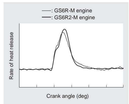
**Fig. 4 Comparison of heat release rates**
