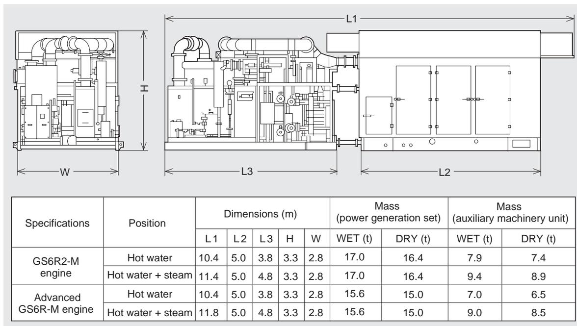
**Fig. 5 External view and dimensions of co-generation system**
