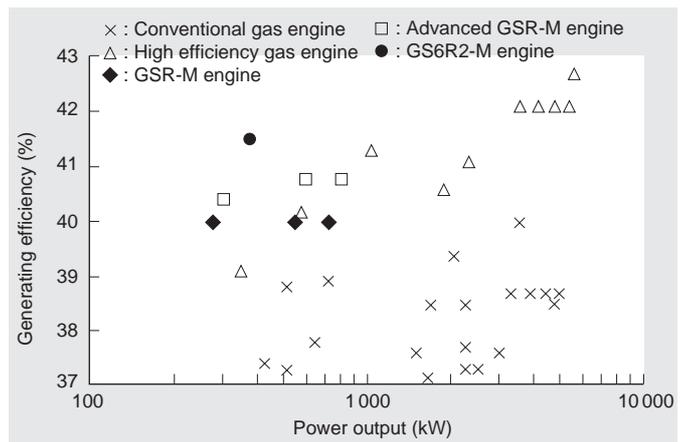
Fig. 2 Relation between generating efficiency and power output in the gas engine
