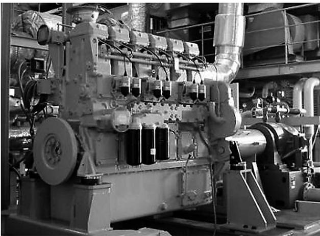
Fig. 1 External view of GS6R2 Miller cycle gas engine
