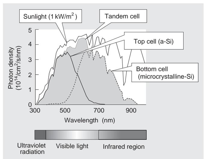
**Fig. 3 Wavelength regions utilized in a tandem PV module**
