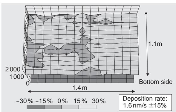
**Fig. 6 Results of deposition of microcrystalline-Si film on 1.4 m x 1.1 m large area substrate**
