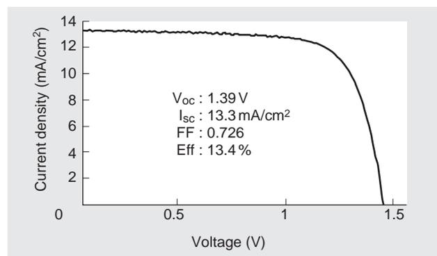
**Fig. 7 Characteristic initial power generation curve for a small area tandem thin film solar cell fabricated with a small area plasma enhanced CVD apparatus**
