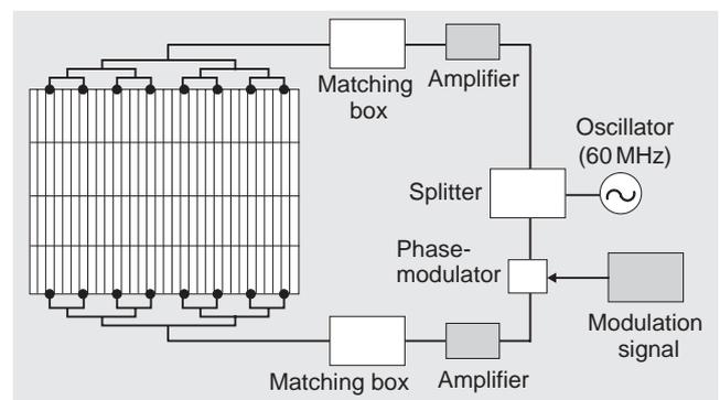
Fig. 1 Conceptual principle of ladder shaped electrode and phase modulation method
