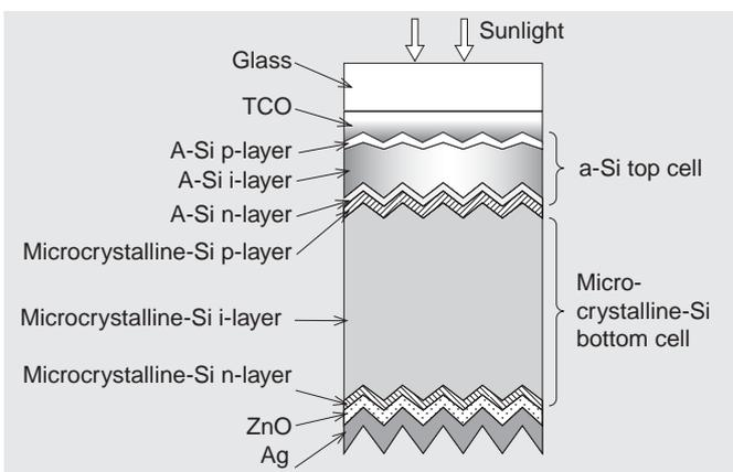
**Fig. 2 Structure of tandem PV module**
