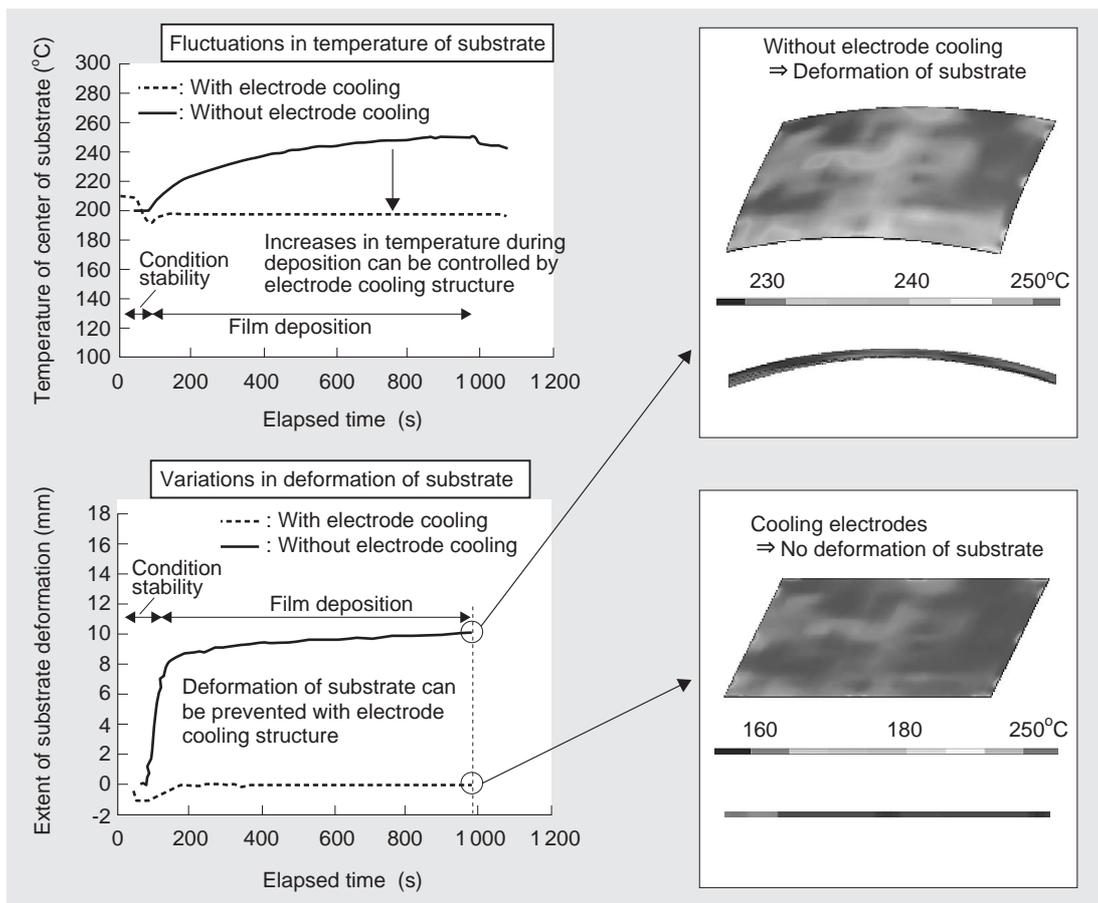
**Fig. 5 Results of analysis of fluctuations in the temperature of the substrate and deformation of the substrate during deposition based on thermal strength coupled analysis**
