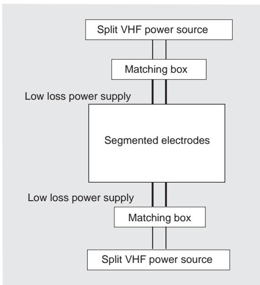
**Fig. 4 Schematic of the electrodes in the large area plasma enhanced CVD apparatus used for deposition of microcrystalline-Si**
