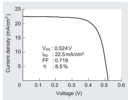
**Fig. 8 Initial power generation characteristics of microcrystalline-Si single junction solar cell on a large area substrate**
