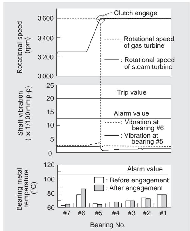
**Fig. 9 Operation of turbine using SSS clutch**
