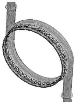
**Fig. 5 Scroll type steam inlet**
