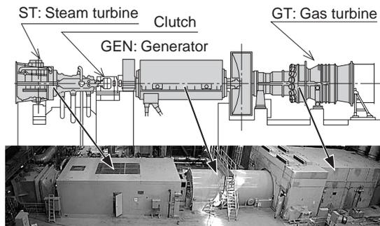
**Fig. 7 Turbine shaft arrangement applying SSS clutch**
