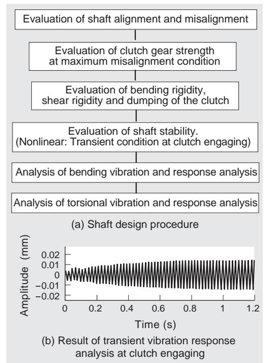
**Fig. 8 Design of shaft system including SSS clutch**
