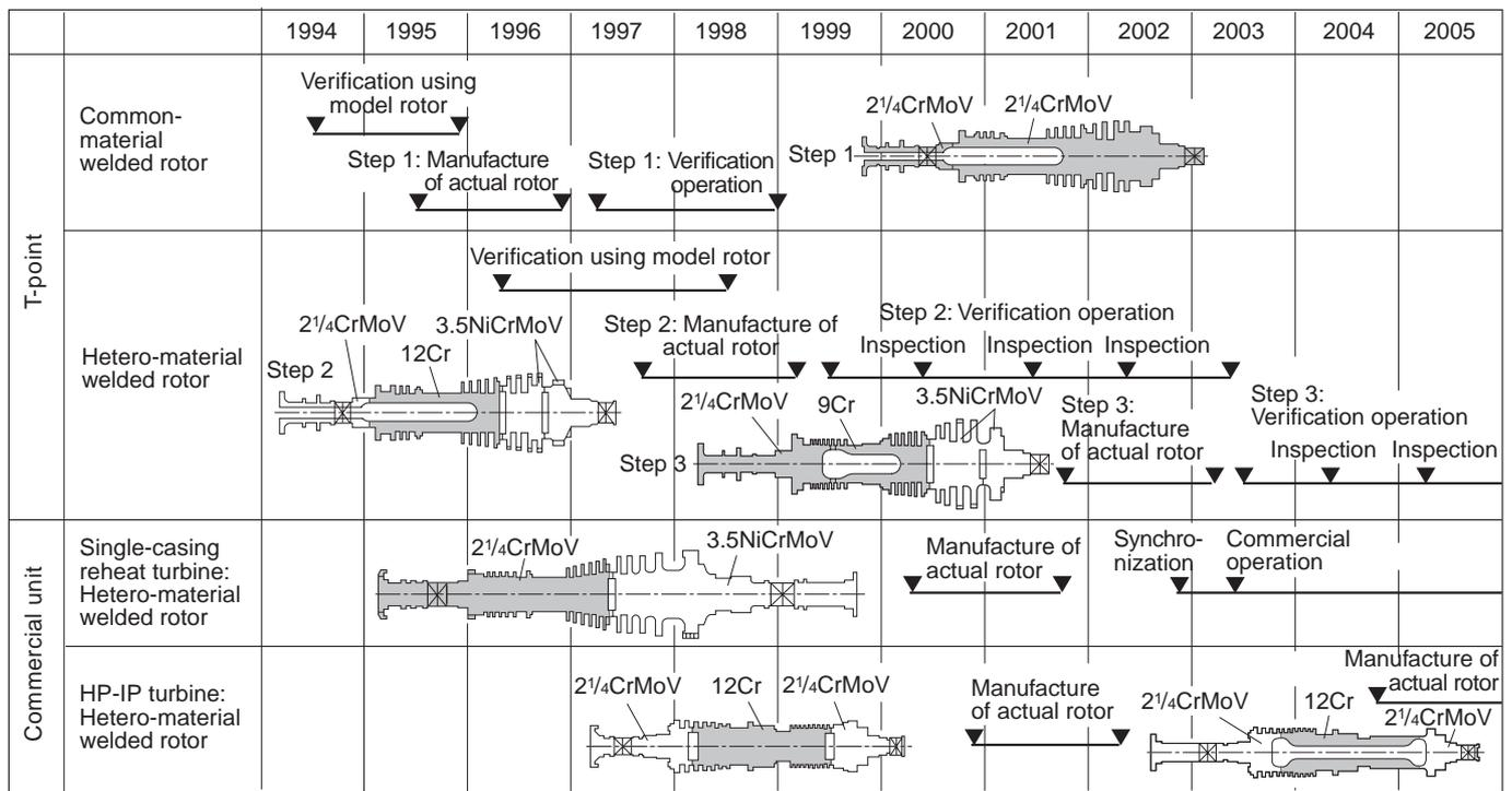
Fig. 3 Application of welded rotor to actual turbine
