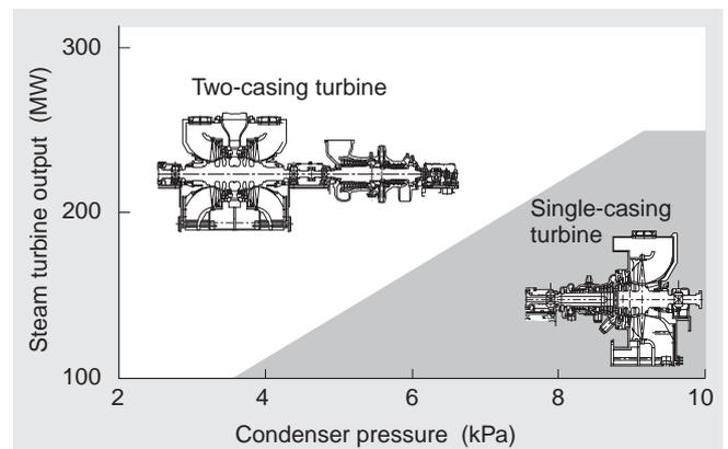
**Fig. 1 Steam turbine capacity and casing arrangement**
