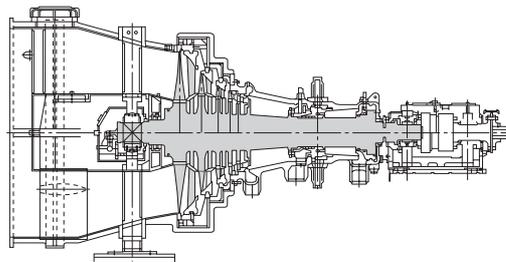
**Fig. 6 Large-capacity axial-exhaust single-casing reheat turbine**
