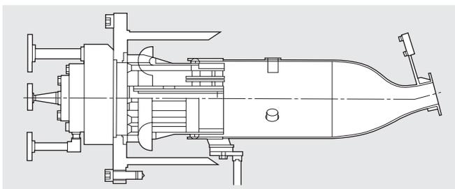
Fig. 3 Examination schematic of 1700°C diffusion type combustor
