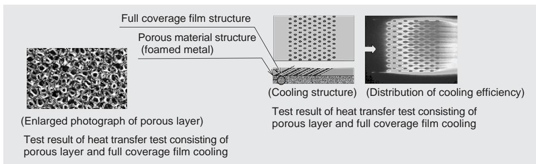
Fig. 7 Example of transpiration cooling system
