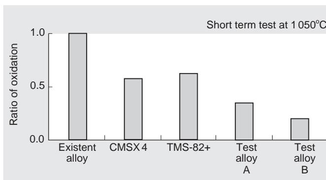
**Fig. 11** Atmospheric oxidation test results for each alloy
