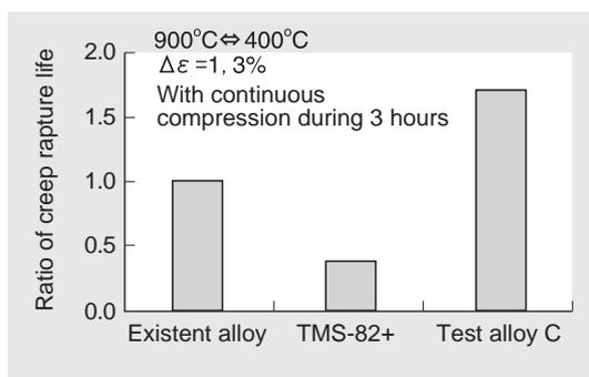
**Fig. 10** Thermal fatigue test result for each alloy
