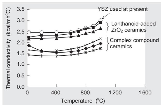
**Fig. 14** Results of measurements of thermal conductivity of trial manufactured sintered ceramics
