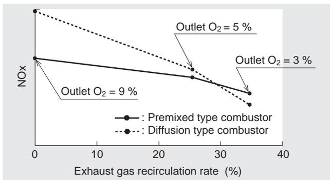
Fig. 5 Estimation of emitted NOx by CFD
