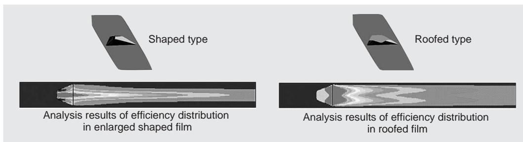
Fig. 8 Analysis result of new type film cooling
