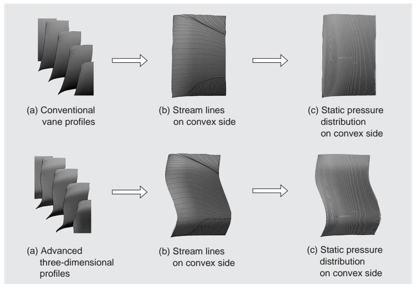
Fig. 20 Comparison between conventional stationary vane and newly designed three-dimensional stationary vane
