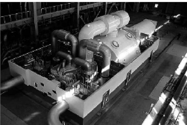
Fig. 5 600 MW steam turbine of Hirono No. 5
