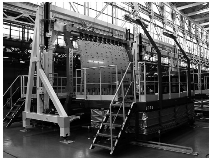
Fig. 6 Common support fixture and work step with lifting function
