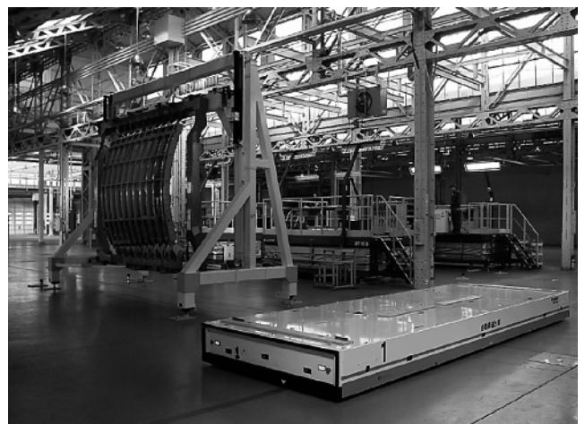
Fig. 2 Automatic guided vehicle Automatic handling is possible.
