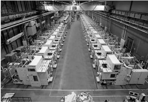
**Fig. 7** Layout of machining line for leading U.S. automobile manufacturer (Rough machining line using several machining centers).
