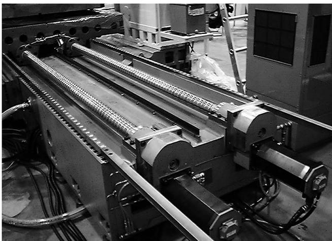
**Fig. 1 X-axis twin ball screw**
