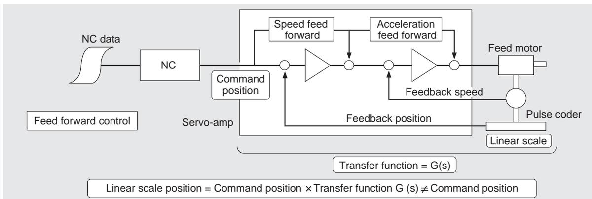
Fig. 2 Block diagram of feed forward control
