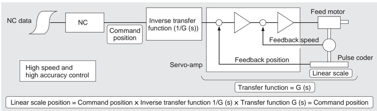
Fig. 3 Block diagram of high speed and high accuracy control (FM control)
