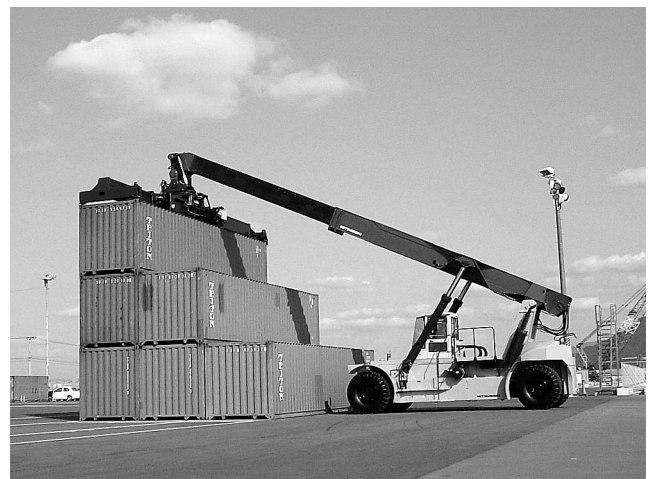
Fig. 2 View of reachstacker at work
