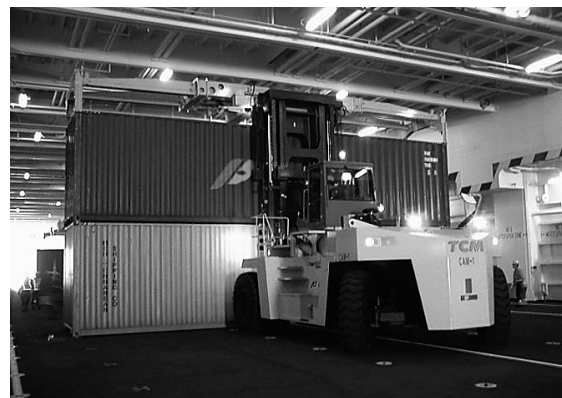
Fig. 2 Loading and unloading cargo with the "Top Lifter" cargo forklift
