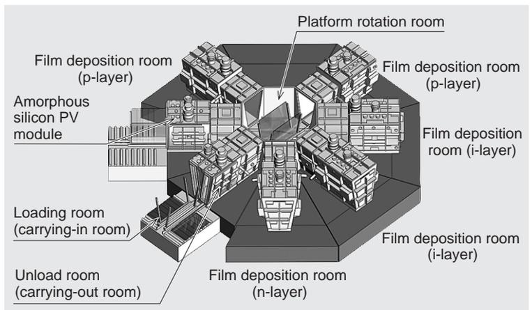
**Fig. 4 Five-room star layout large-area high-rate plasma CVD facilities**
