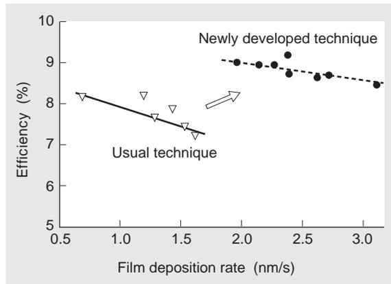
**Fig. 3 Microcrystalline silicon film high-quality and high-rate formation**
