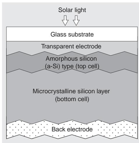
**Fig. 1 Amorphous Si/microcrystalline Si tandem PV module structure**
