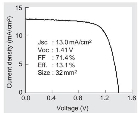
Fig. 7 Initial generation characteristics of tandem cell
