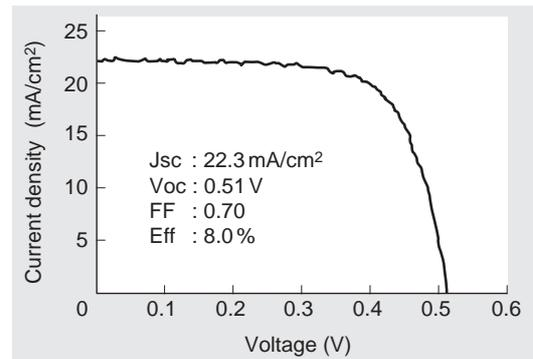
Fig. 12 Power generation characteristics of micro-crystalline Si cell obtained by high-rate film deposition using VHF plasma
