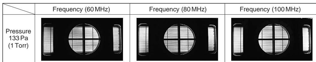
**Fig. 10** SiH<sub>4</sub>/H<sub>2</sub> plasma emission distribution at phase modulation
