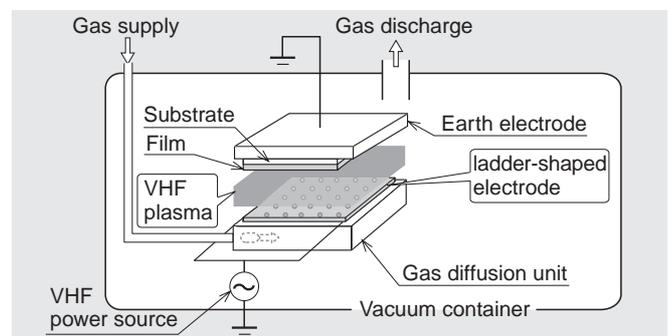
Fig. 1 Concept of VHF plasma CVD using ladder-shaped electrode
