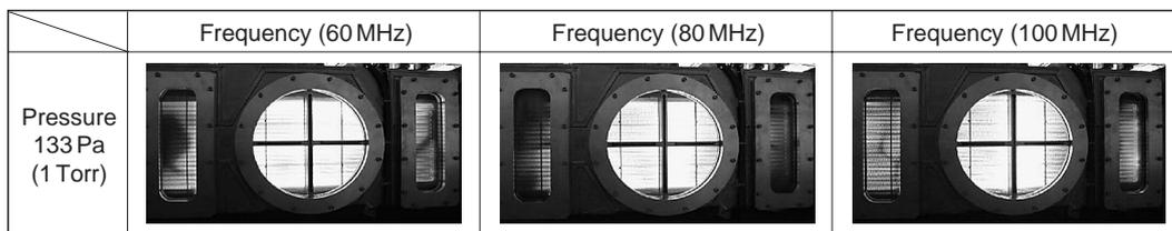
**Fig. 9** Plasma frequency characteristics of SiH<sub>4</sub>/H<sub>2</sub> plasma emission distribution
