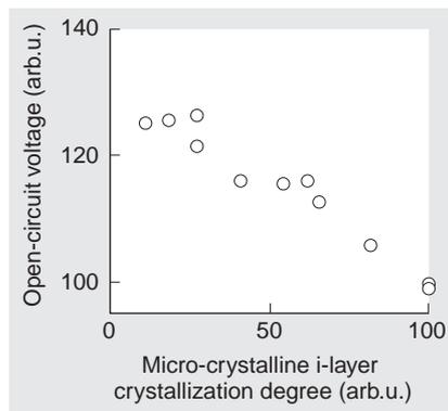
Fig. 3 Dependence of micro-crystalline Si single cell open-circuit voltage on i-layer crystallization degree
