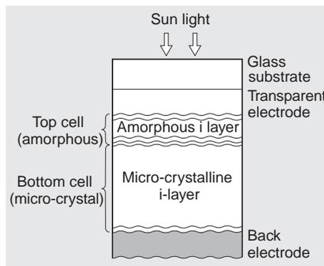
Fig. 6 Structure of tandem cell
