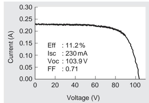
**Fig. 11** Initial generation characteristics of 40 cm x 50 cm tandem module
