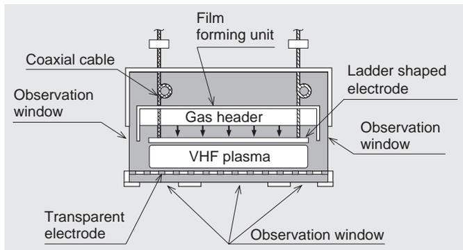
**Fig. 8** Concept of VHF plasma visualization device (unit)
