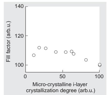
Fig. 4 Dependence of micro-crystalline Si single cell fill factor FF on i-layer crystallization degree
