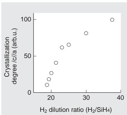
Fig. 2 Dependence of micro-crystalline i-layer crystallization on H<sub>2</sub> dilution ratio
