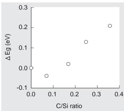
Fig. 5 Dependence of micro-crystalline SiC band gap change on C/Si ratio
