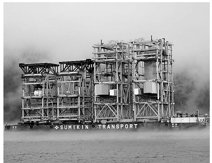
Fig. 5 Transport of boiler module
