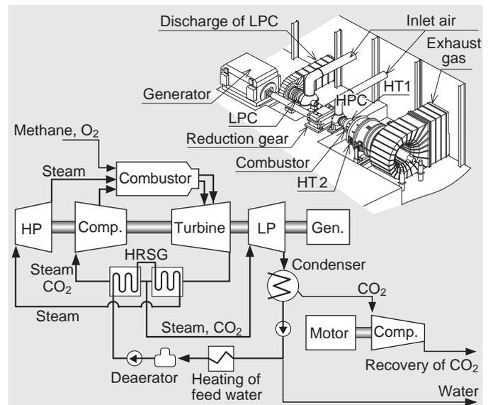
Fig. 10 CO<sub>2</sub> closed cycle
