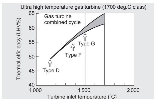
Fig. 4 Technical challenges to higher combustion temperature
