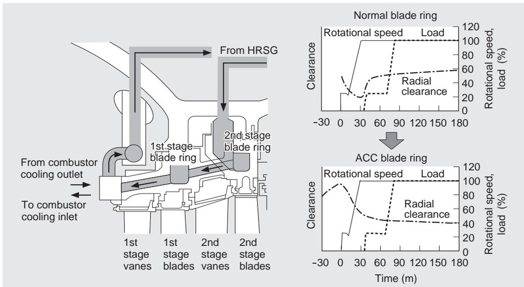
Fig. 3 Blade tip active clearance control (ACC)
