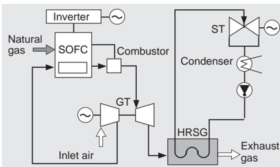
Fig. 8 SOFC + GT combined system
