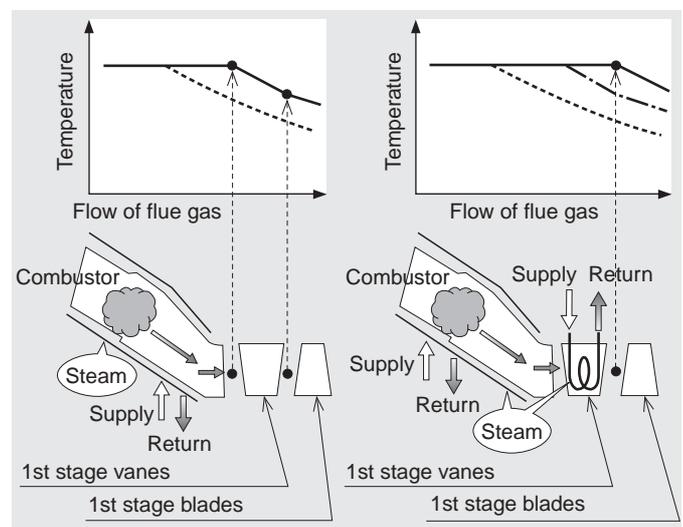
Fig. 1 Steam cooled combustor system
