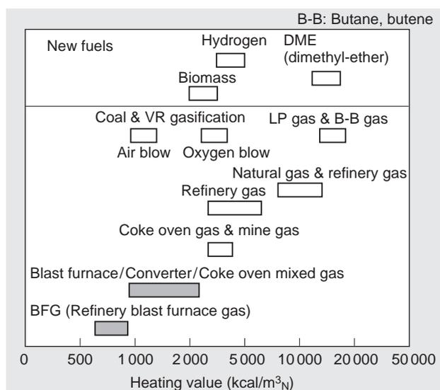
Fig. 5 Diversification of gas turbines fuels
