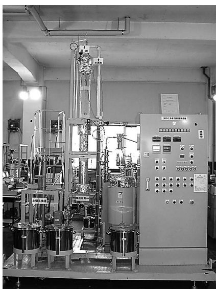
Fig. 3 Actual soil sample testing facility
