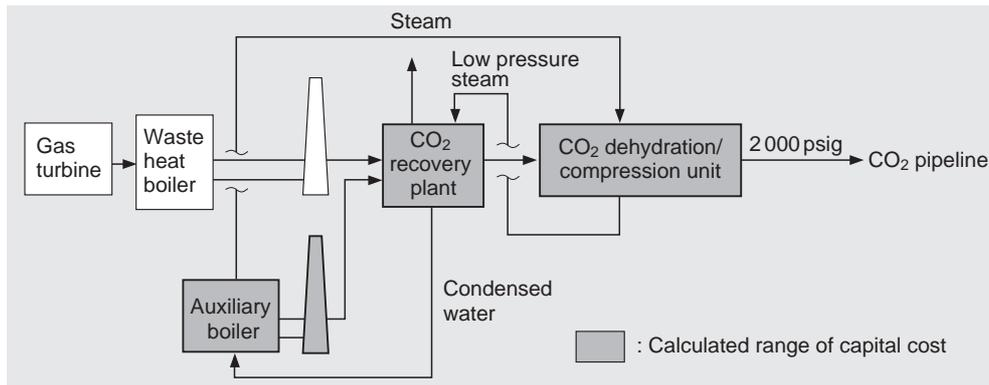
Fig. 3 Gas turbine case
