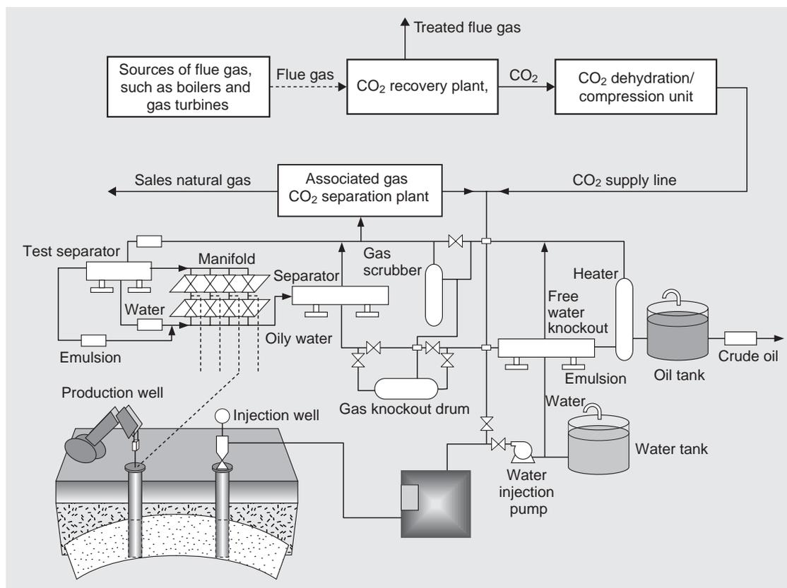
Fig. 1 Concept of overall system for CO<sub>2</sub> EOR
