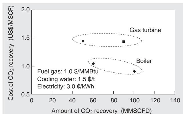
Fig. 4 Relation between CO<sub>2</sub> recovery cost and CO<sub>2</sub> recovery capacity in the flue gas CO<sub>2</sub> recovery plant
