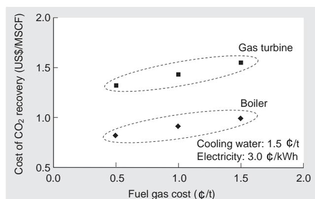
Fig. 5 Relation between CO<sub>2</sub> recovery cost and fuel gas cost
