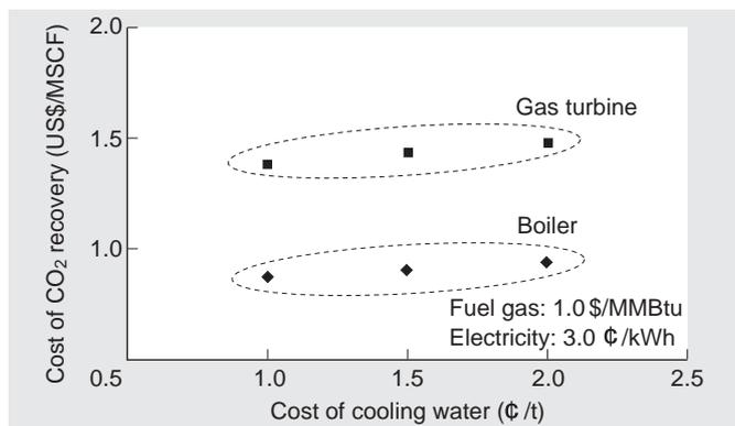
Fig. 6 Relation between CO<sub>2</sub> recovery cost and cooling water cost
