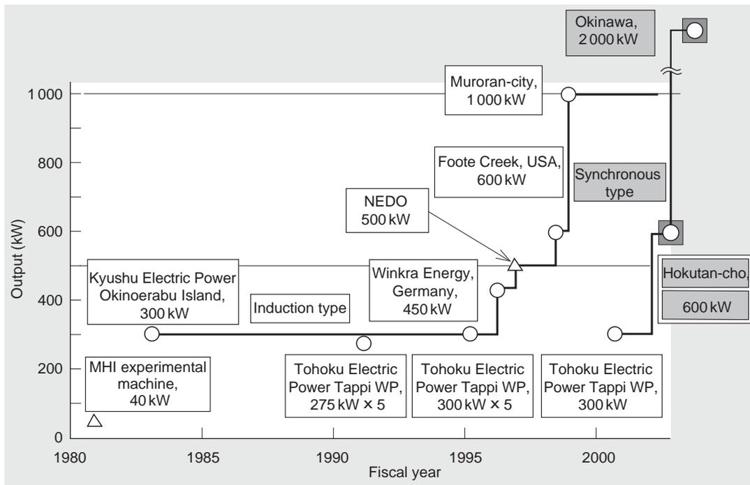
**Fig. 3 History of development of MHI wind-turbine power generator**
