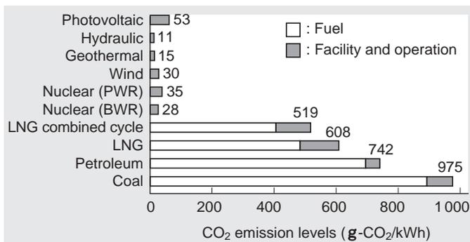
Fig. 1 CO<sub>2</sub> emission levels of several power generation systems
