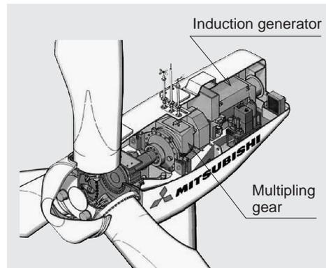
**Fig. 5 Structure of MWT-1000A**
