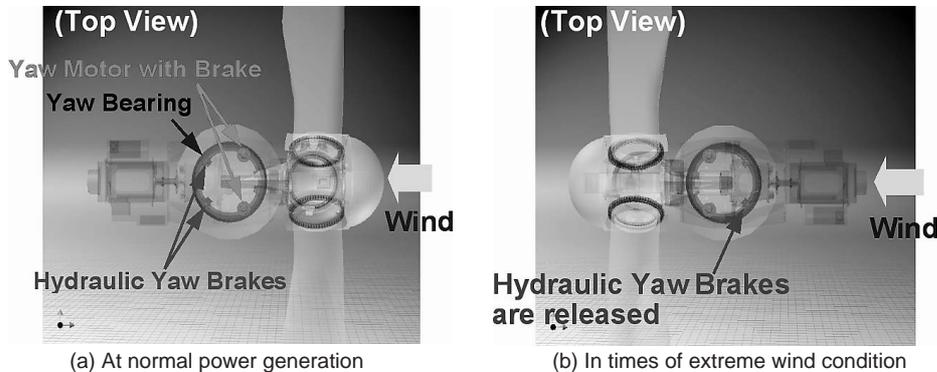
**Fig. 9 Concept of Smart-Yaw operation**, with (a) indicating the wind turbine faced up wind direction for operation by using yaw-motor and hydraulic yaw brake at normal power generation while (b) indicating the wind turbine set to face naturally down wind direction by releasing hydraulic yaw brake in times of extreme wind condition.
