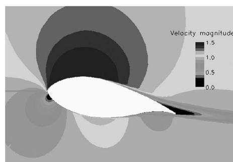
Fig. 6 Flow around the optimized airfoil
