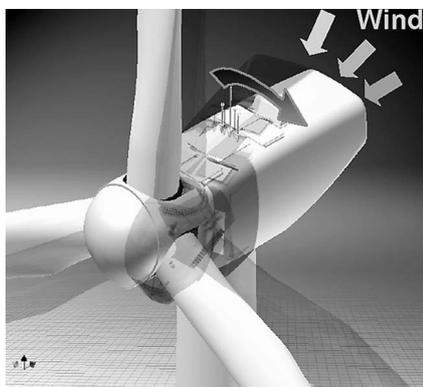
**Fig. 8 Down wind directivity of wind turbine**
