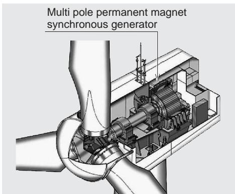
**Fig. 4 Structure of MWT-S2000**
