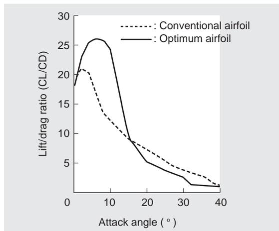
**Fig. 7 Measured values of aerodynamic characteristics of conventional and optimum type airfoils**
