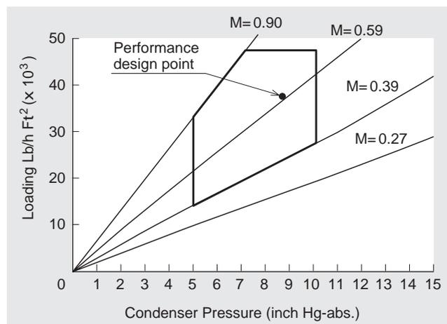
Fig. 3 Design specification range of low-pressure blade
