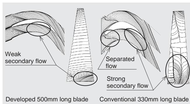
Fig. 5 Results of three-dimensional viscosity fluid analysis
