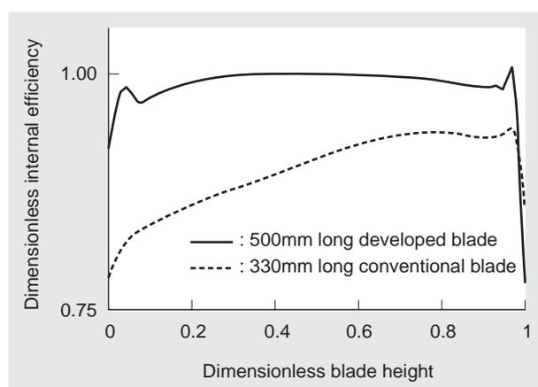
Fig. 6 Evaluation of performance of low-pressure blades (three stages) (Comparison with conventional blade)
