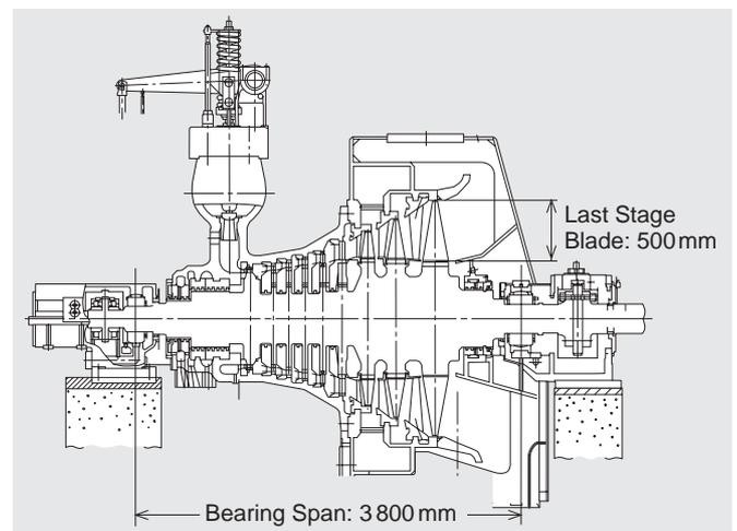
Fig. 2 Plan of steam turbine for GTL plant
