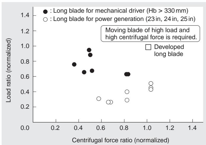
Fig. 1 Relation between centrifugal force and load acting on blade (comparison with conventional blades of MHI)
