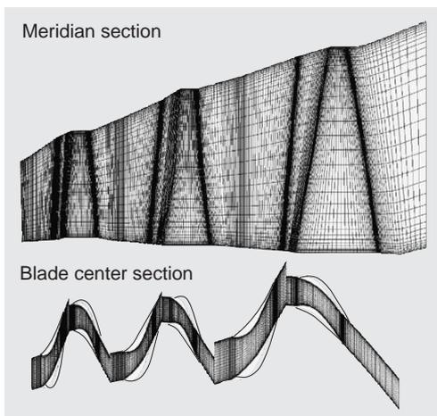
Fig. 4 Calculation grid of three-dimensional viscous flow analysis
