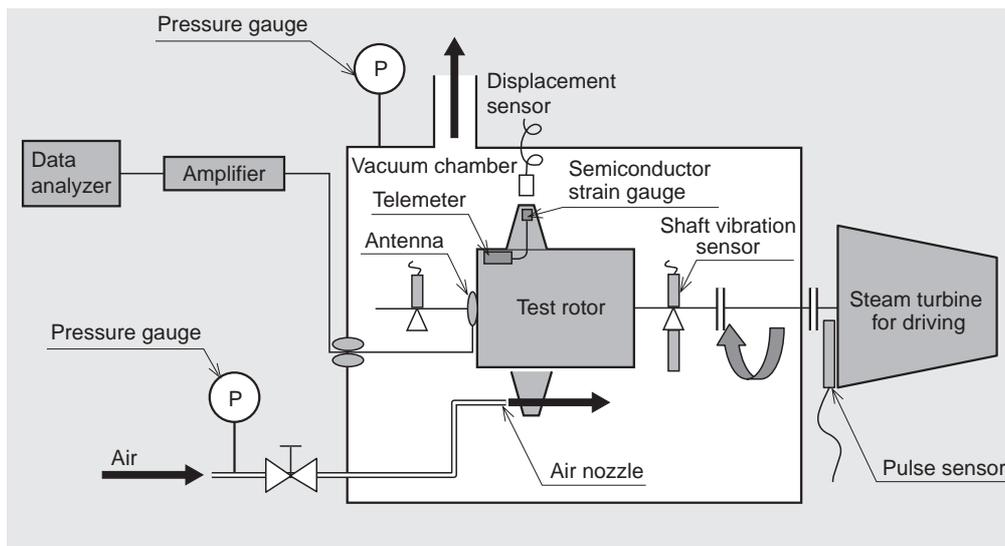
Fig. 12 Configuration of measuring equipment of rotation vibration test
