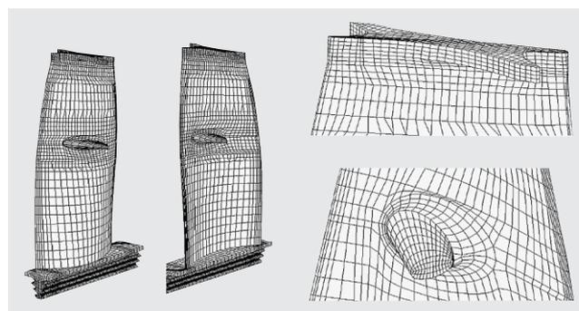
Fig. 7 Finite element model of L-0 stage
