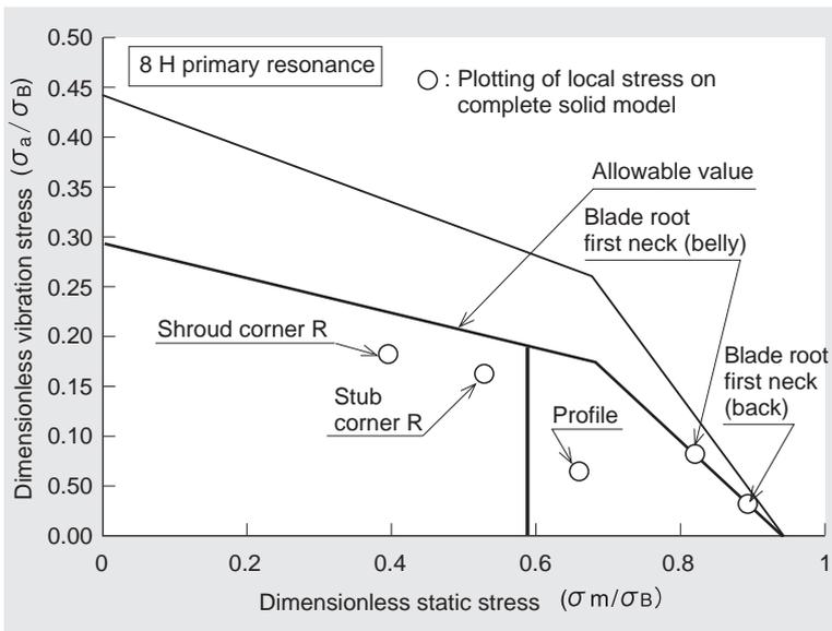
Fig. 10 Goodman diagram of L-0 stage
