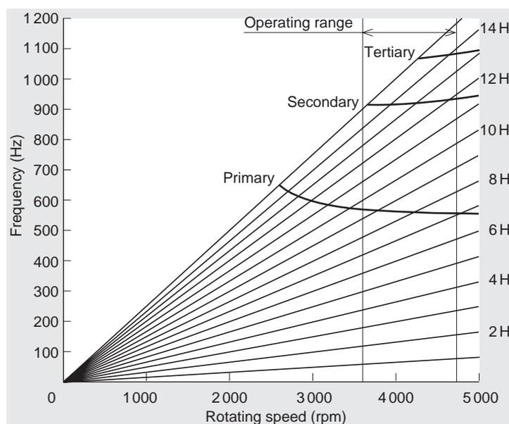
Fig. 9 Campbell diagram of L-0 stage (result of analysis)
