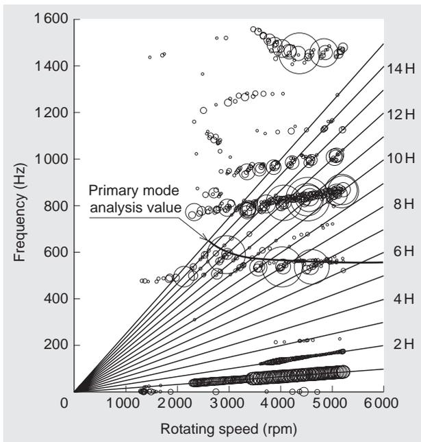
Fig. 13 Campbell diagram of L-0 stage
