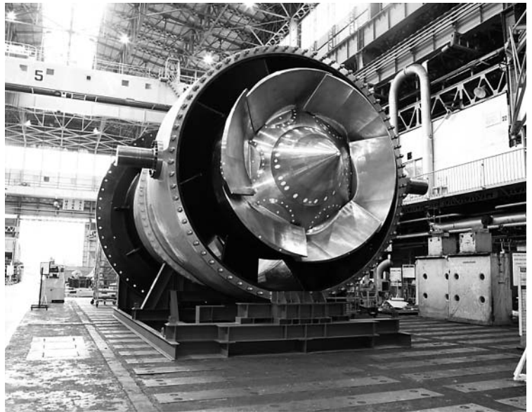
Vertical shaft diagonal flow type pump and vertical shaft axial flow type pump (used for preventing flood, sewage system and circulating water in power plant)
