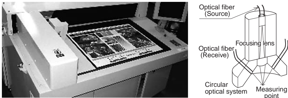
Fig. 2 Examples of application (1) Control console for color control system, (2) small color sensor with optical system.
